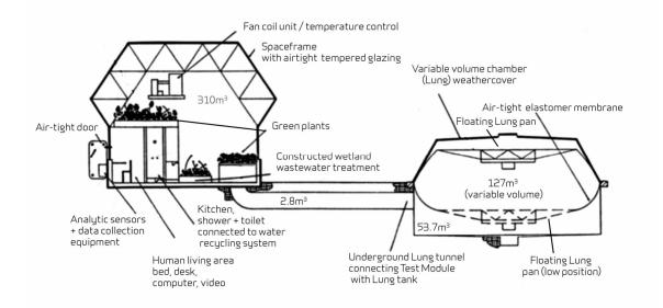
Figure 3. Schematic of the Biosphere 2 Test Module. The engineering and ecological research program included air-tight sealing techniques, the feasibility of a variable volume chamber to alleviate stress on the structure, the efficacy soil bed reactors, constructed wetlands for wastewater recycling and the response of a variety of plants and human beings in closed ecological system conditions.
