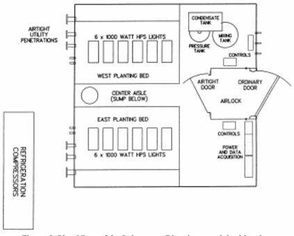
Figure 5. Plan View of the Laboratory Biosphere modular biosphere (Dempster et al, 2004)
