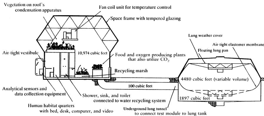
**Figure 1.** Schematic of Biosphere 2 test module showing its configuration during a series of human enclosure experiments conducted from 1988 to 1990. Its main structure is approximately 7 m on a side by 8 m tall, with a variable volume of approximately 480 m<sup>3</sup>.
