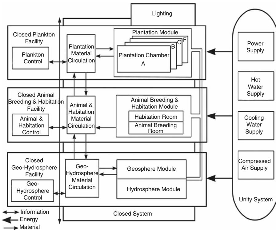
**Fig. 11.19.** System Configuration of Closed Ecology Experiment Facilities (CEE) (73).
