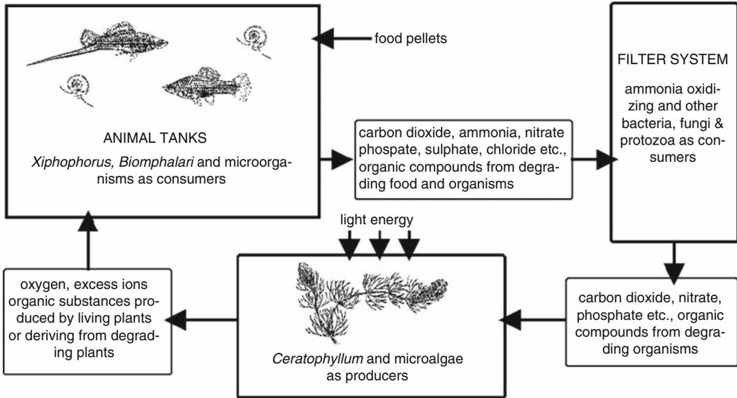
**Fig. 11.15.** Functional relationships of the basic components of the C.E.B.A.S. The animal tank is combined with an aquatic plant bioreactor and with a bacteria filter, which contains ammonia oxidizing bacteria (65).
