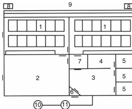
**Fig. 11.13.** BIOS – 3. Design of the Bios-3 experimental system. 1 – phytotrons; 2 – algal cultivator compartment; 3 – living quarters; 4 – kitchen–dining-room; 5 – cabins; 6 – toilet lock; 7 – vestibule; 8 – pumps of the cooling system for light sources; 9 – watering collector of the heat exchange wall of phytotrons; 10 – pressurization compressor; 11 – bacterial filter (16).
