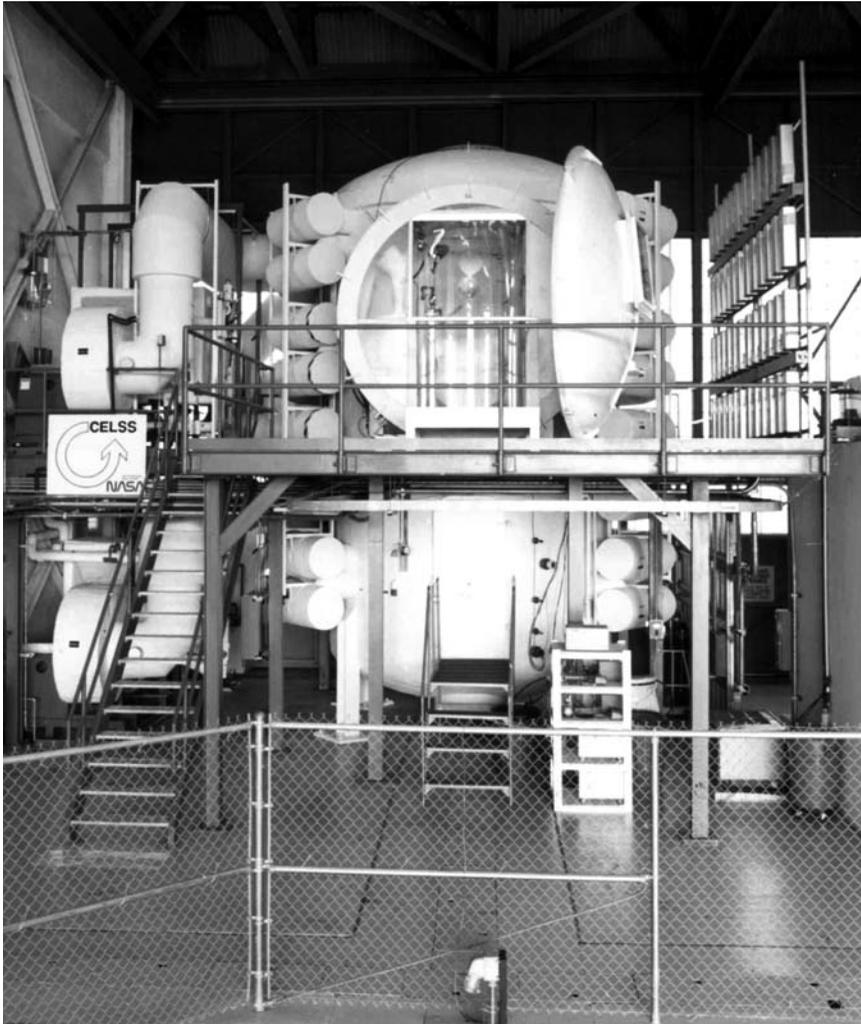
**Fig. 11.1.** Breadboard Plant Chamber at Hangar L at KSC, FL (front view, 1986). The chamber provided a closed atmospheric volume of about  $113 \text{ m}^3$  (including air ducting) with  $20 \text{ m}^2$  of crop growing area. External nutrient solution tanks were not in place at the time of this photo (12).
