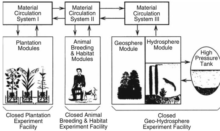
**Fig. 11.18.** Closed ecology experimental facility (CEE) (From Closed Ecology Experiment Facilities (CEE) (73).
