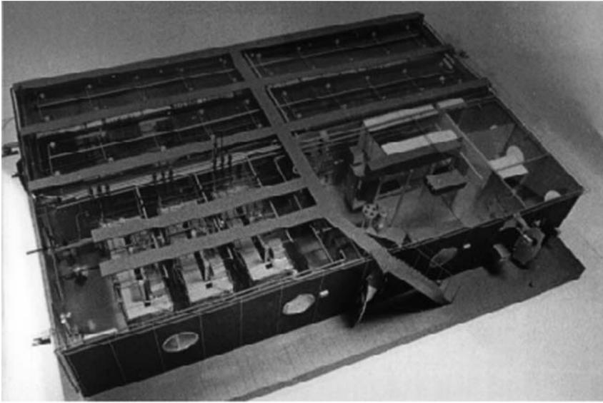
**Fig. 11.12.** General view of the Bios-3 (model with transparent roof). Front left – algal compartment; right – crew compartment; back – two higher-plant compartments. Light sources are on the roof of installation. Ladders and gangways on the roof are for servicing light sources. On the front wall, to the right – entrance of one of crew’s cabins. To the right and left of it – airlocks for passing tools, chemical reagents, and other things in and out (16).
