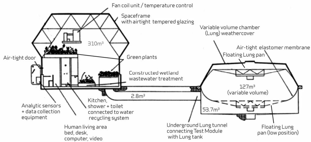
Figure 3. Schematic of the Biosphere 2 Test Module. The engineering and ecological research program included air-tight sealing techniques, the feasibility of a variable volume chamber to alleviate stress on the structure, the efficacy soil bed reactors, constructed wetlands for wastewater recycling and the response of a variety of plants and human beings in closed ecological system conditions.
