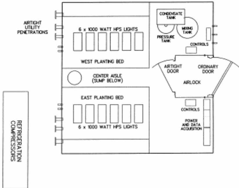
Figure 5. Plan View of the Laboratory Biosphere modular biosphere (Dempster et al, 2004)
