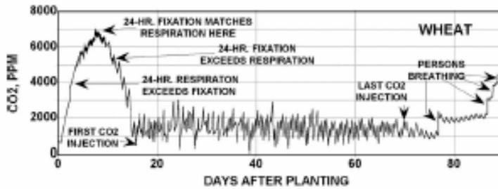
Figure 6. Atmospheric carbon dioxide dynamics in the Laboratory Biosphere during a 2003 experiment with wheat (Dempster et al, 2005). Early rise in CO<sub>2</sub> was from soil respiration exceeding uptake by young plants; the rise at the end reflected human respiration during the process of wheat harvest operations. During the main growing period, CO<sub>2</sub> was injected as needed and drawn down during hours of light by the crop.
